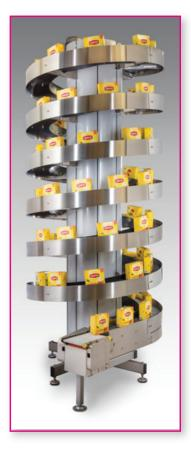
Ryson Spiral conveyors move products vertically within a very small footprint, and have a very high throughput. This ultimately reduces the floor space requirements while allowing access to overhead space.
