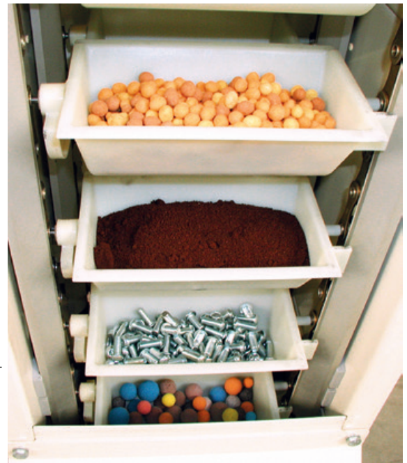
The swinging pendulum design allows for a gentle and reliable transport, and transitions from horizontal to vertical motion without disturbing the load.
