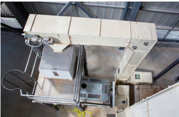
Fully enclosed Bucket Elevators help mitigate foreign debris and help with product integrity
