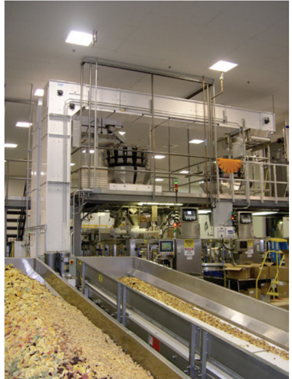
Bucket Elevators are often used to transport ingredients to a top loaded checkweigher or hopper.
