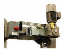
Pre-Wired motor disconnect switch, Chain Tension and Motor Overtorque sensors pre-wired to a common terminal enclosure
